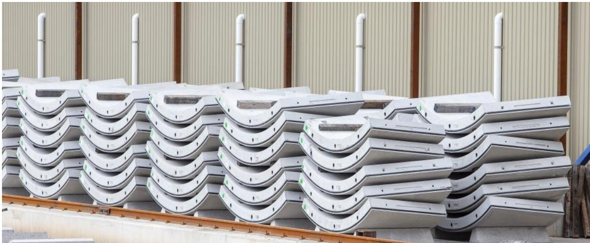
Figure 6: Pre-Cast Concrete Tunnel Segments at the Marrickville Dive Site
