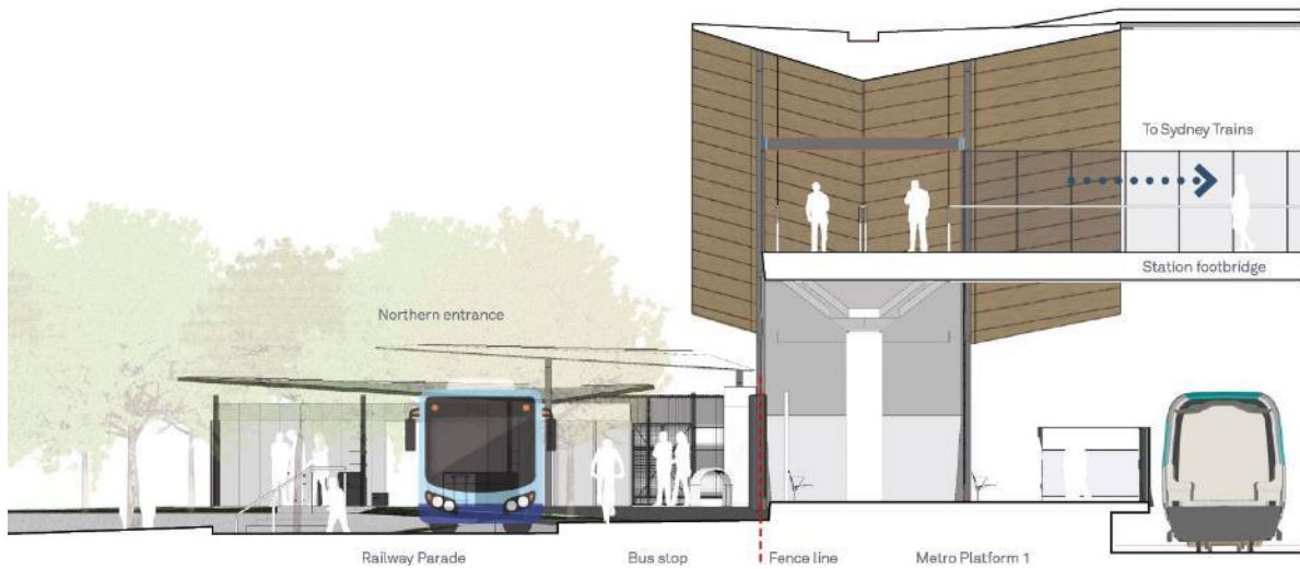
Figure 6.1.2: Northern plaza interchange section
