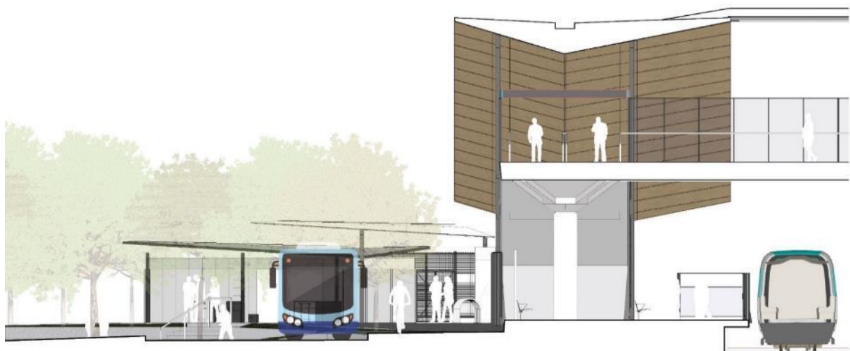
Figure 4.1.2: Sectional diagram showing bus and Metro interchange on Railway Parade
