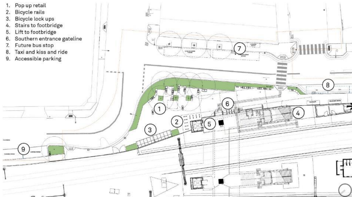
Figure 6.1.8: Sydenham station southern entrance plan
