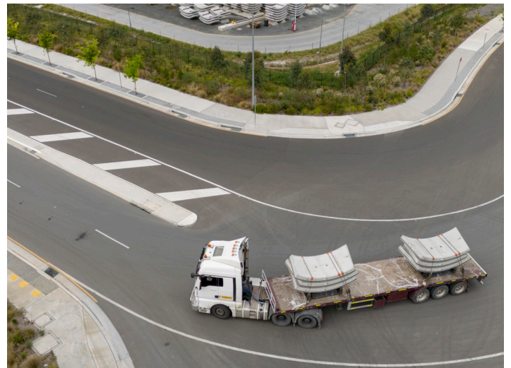
Concrete segment delivery from Eastern Creek Precast Facility.
